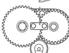
Crankshaft Locking Tool is used to set the crankshaft timing position during both removal and replacement of the timing belt. The crankshaft is first turned to TDC on N0.1 cylinder, checking the timing marks on the camshaft sprocket hubs are aligned.
