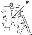
Support Guides. Some cars require the front panel to moved forward to enable access to the engine.
