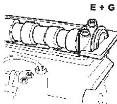
**Injection Pump Pulley Locking Pin** is 15,4mm. diameter and is used on engines having a one piece Injection Pump Sprocket.
