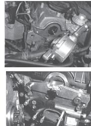
M5 x 55mm. Stud and Nut. This is used to apply pressure to the tensioner plunger to release the tension from the timing belt.
