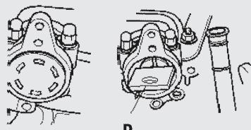
**Camshaft Setting Bracket** is used to set the correct timing position of the camshaft. The centre part of the bracket fits into the slotted end of the camshaft. The ends of the bracket locate on the cylinder head. The correct alignment is achieved by placing equal thickness of shim/feeler gauge between both ends of the bracket and the cylinder head.
